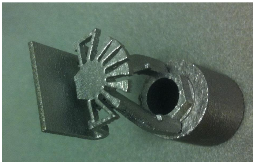
Figure 7 A photo of a 1:4 T-Rex nozzle that is made of steel.
