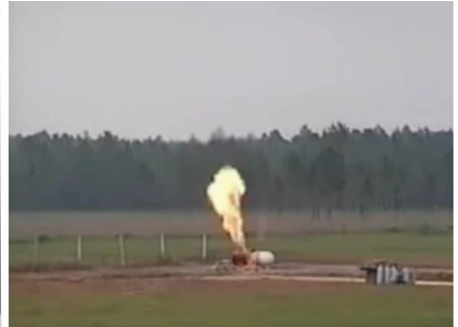
Jet, BLEVE and fireball ( Superheat temperature )
