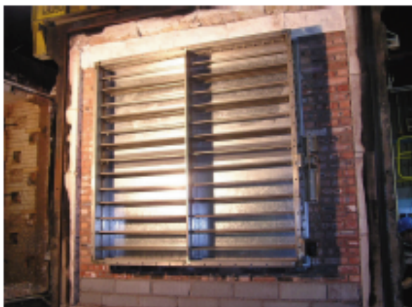
Figure 7 Damper assembly after the 250 °C for 2 hours fire test. The furnace is at the background on the left
