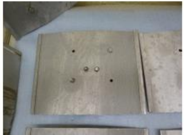
Figure 5 Results obtained on a specimen, which was treated. Almost no corrosion on the material and on the bolt is observed
