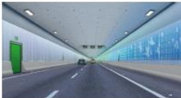
Figure 2 Drawing of the southbound (outer) road tunnel tube with safety and technical equipment
