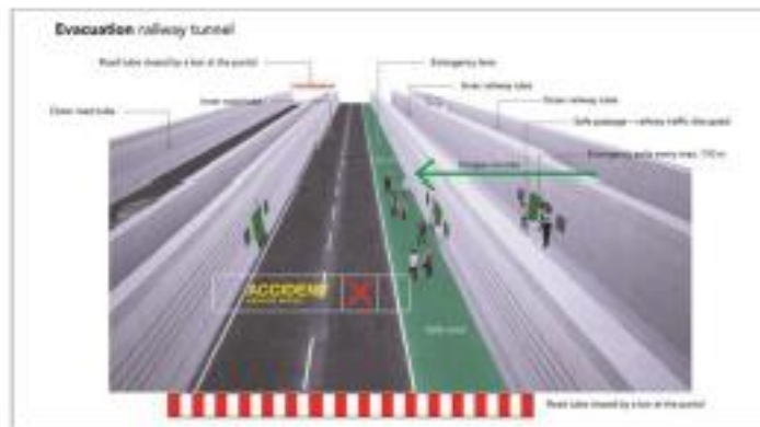
Figure 8 Escape concept for the railway tunnel to the inner road tunnel tube
