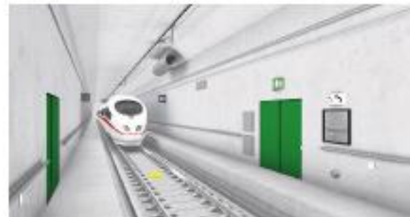
Figure 3 Drawing of the inner rail tunnel tube with safety and technical equipment
